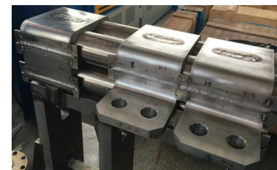
Figure 9. ELM_07, ELM_10 and VS_02 bracket after integration
