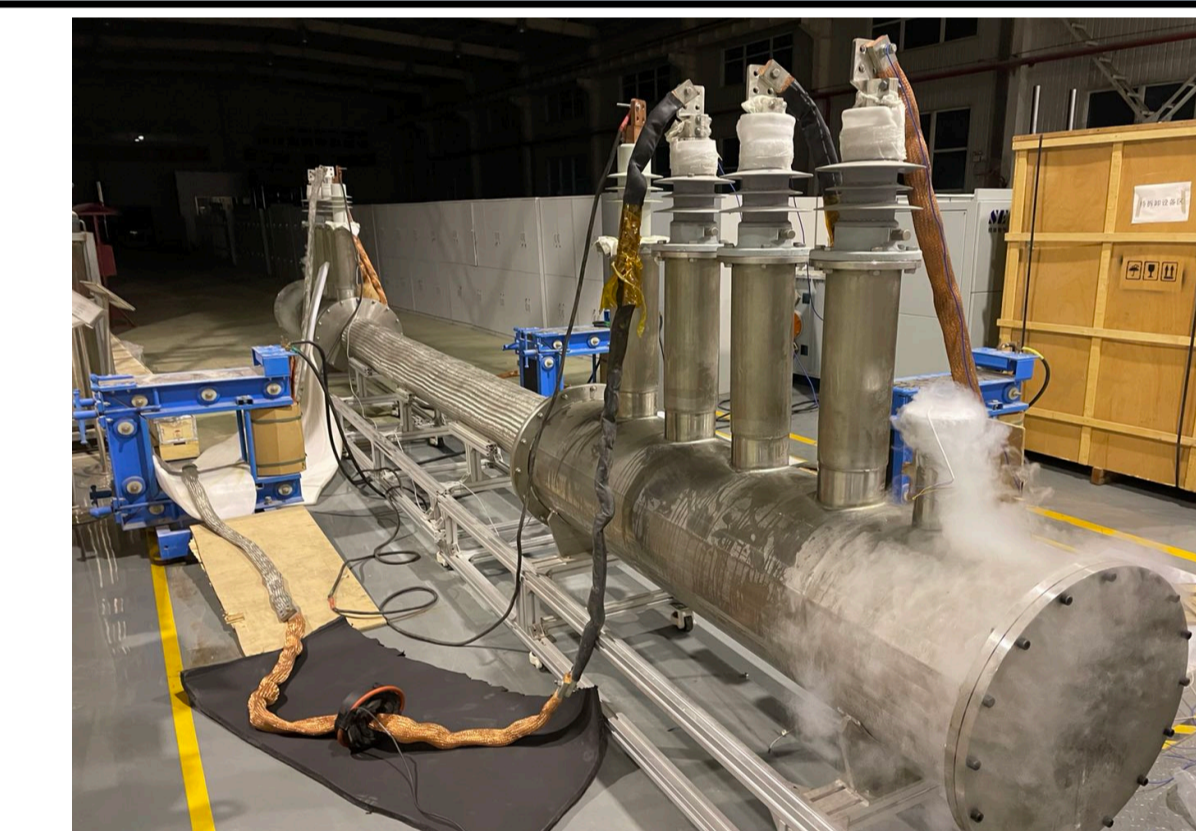
Fig. 6 experiment photo of tri-axial HTS cable
