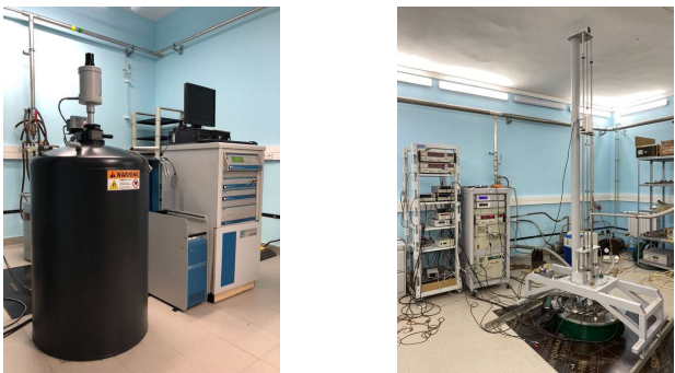
Measurement systems used in this study, enabling magnetic fields up to 9 T, PPMS (left), and 21 T, Cryogenic (right), in the 0.3-300 K temperature range.
