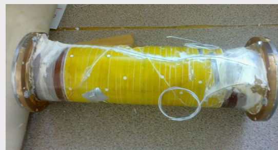
The solenoid after vacuum impregnation with epoxy filled with Al_2O_3 powder.
