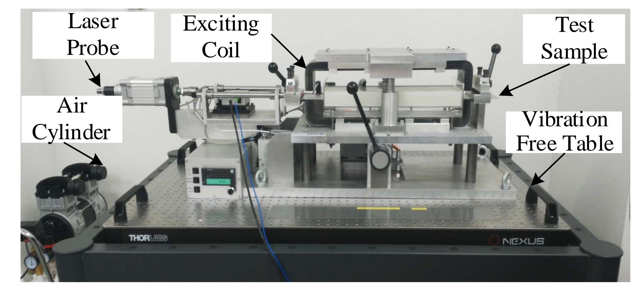
Fig. 2. measurement system of magnetization and magnetostriction
