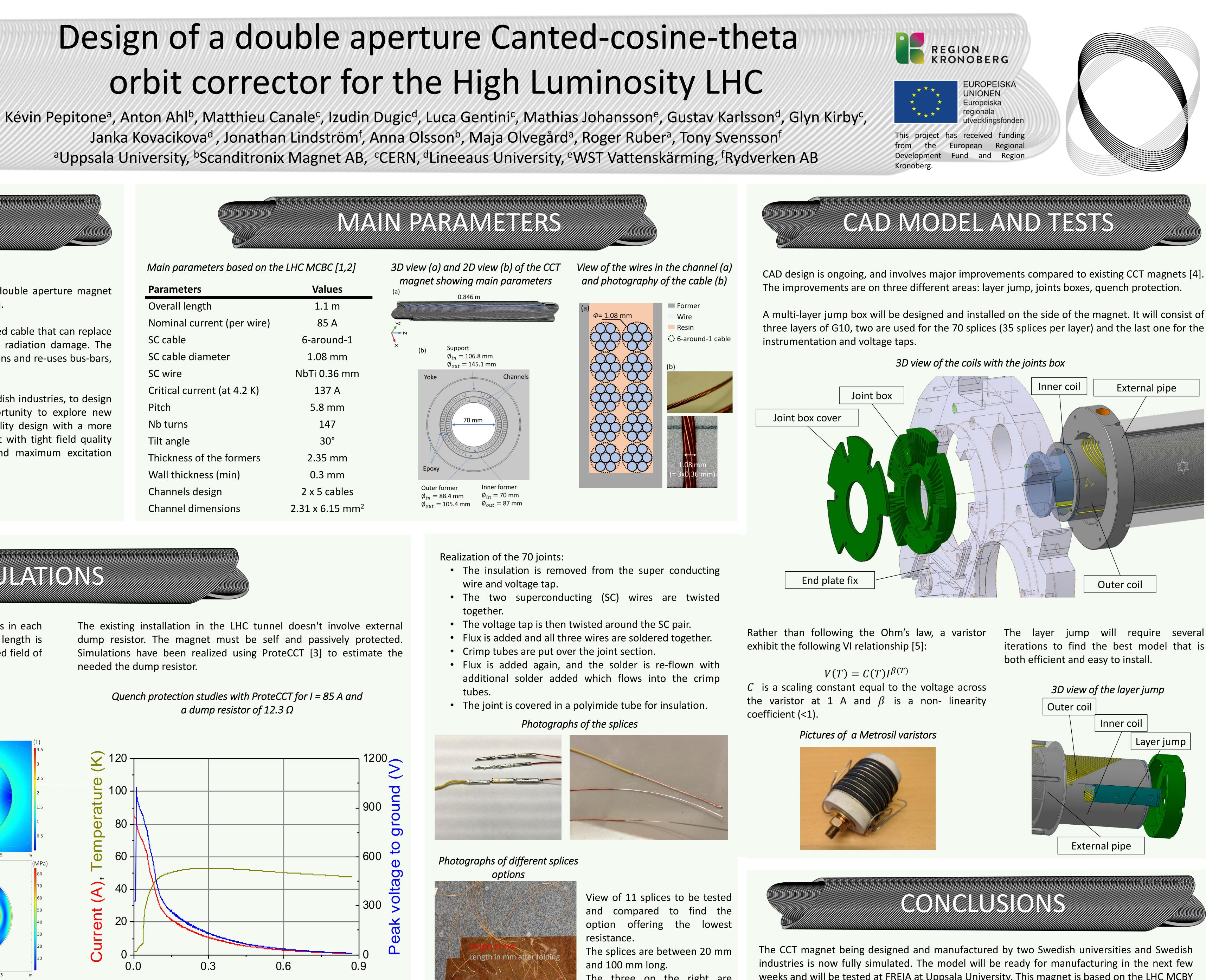
The existing installation in the LHC tunnel doesn't involve external dump resistor. The magnet must be self and passively protected. Simulations have been realized using ProteCCT [3] to estimate the needed the dump resistor.
