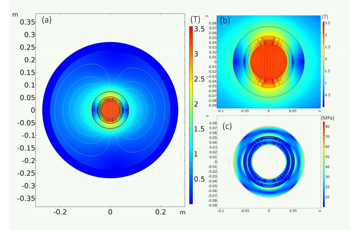
2D view of the magnetic field simulated by COMSOL with iron (a), zoom around the coil (b) and mechanical stress (c)
