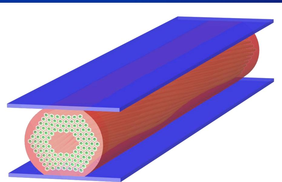
Full detailed 3D geometry of the strand (**no homogenization**).
