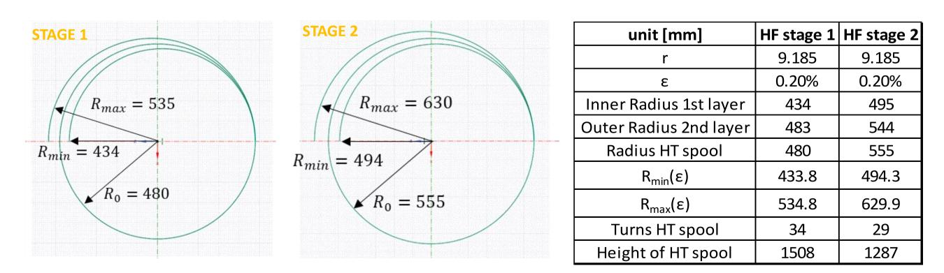
**OPTION 1:** This first analysed option opts for a combined radial and mainly axial reopening of the cable and considers four different spools for the HT, two stages for the HF sub-module, one for the MF and one for the LF sub-module. To analyse the process, the transfer of the first stage of the HF cable is described. This phase leads to complete the first two layers of a CS module starting from the heat treatment spool:
