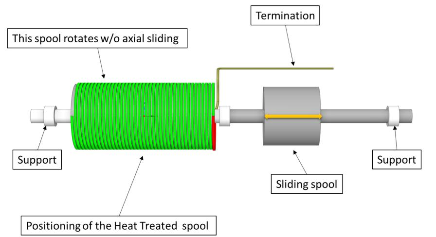
Application of the strain phases A1 and A2. The taping machine is placed on the line and the deformed cable rotates and advances to the entry point of the final spool.
