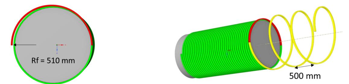
To validate the phases A1 and A2, a FEM model has been defined to evaluate the maximum longitudinal strain. The model comprises a complete turn and a half, and a cylindrical target surface to simulate the spool. One end of the cable is constrained in all directions, while at the other end a radial displacement to 33 mm, and a vertical displacement of 0.75 m are applied.
