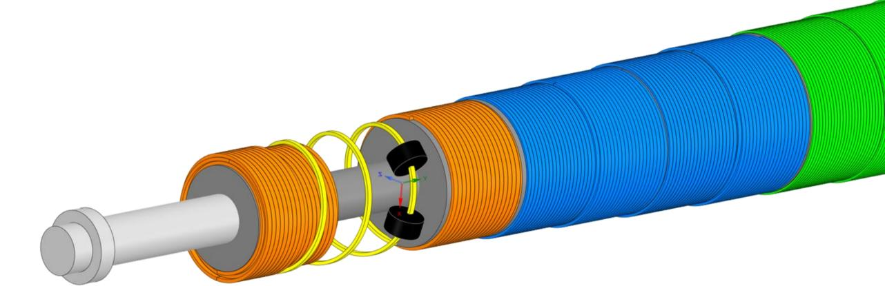
Starting from the spool corresponding to the 1<sup>st</sup> layer of the grade HF (L1), each spool following in the winding system contains a core identical to L1 and n-1 coaxial cylinders of thickness:  $t = d_r(L_i + 1) - d_r(L_i).$
