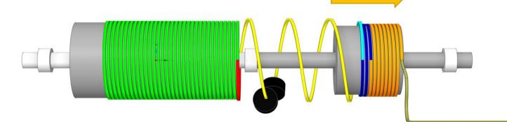
Once the first layer is complete a transition zone with a different pitch switch to the second layer with a distributed jump.
