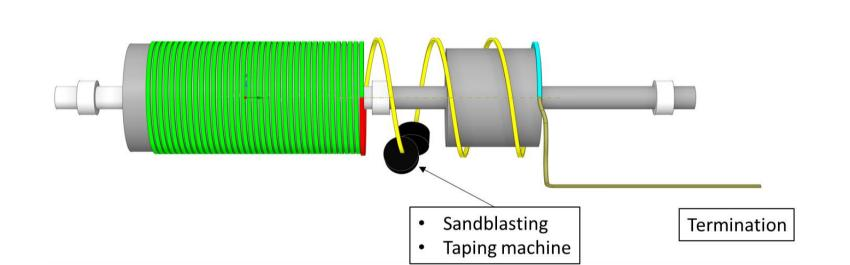
2. The spool rotates and slides axially forcing the cable on the inner radius of the CS.
