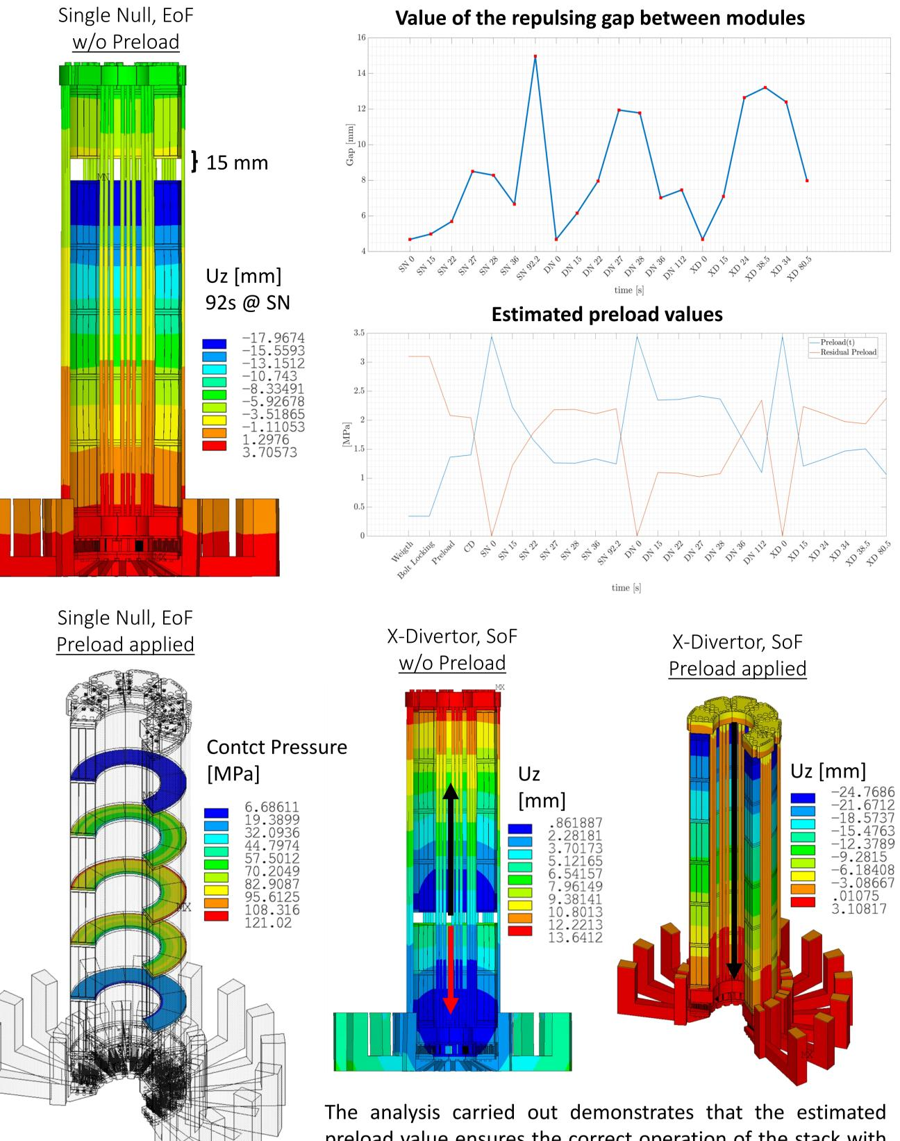
preload value ensures the correct operation of the stack with zero-gap between modules.
