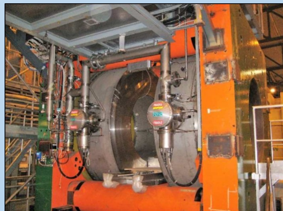
Current M1 and H8 magnets each with 3 T and 1.6 T central fields respectively.
