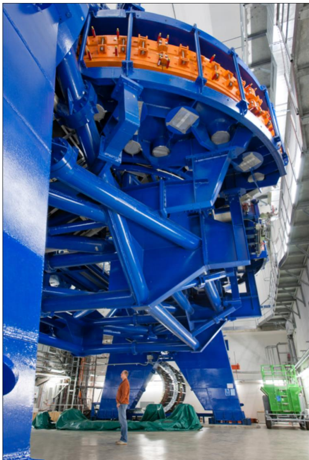
Heidelberg (De)HIT First ion gantry ever Resistive magnets 600 tons rotating 25 m long (2012)
