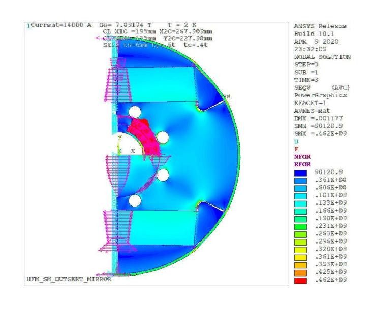
Magnetic flux map and stress distribution in the mirror magnet at 4K - 14kA
