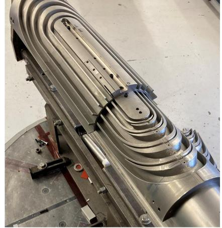
**Coil mandrel on winding table**
