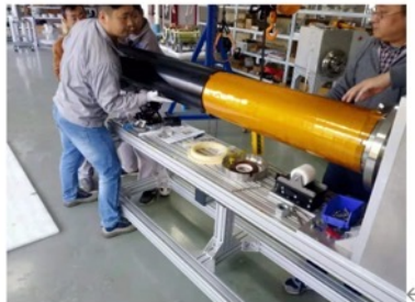
Installation of outer mandrel
