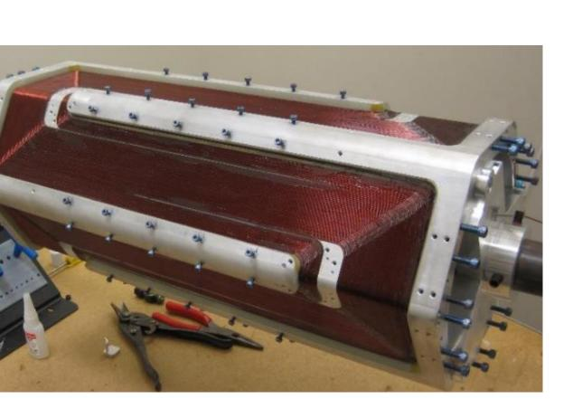
A test dry-winding was performed using copper wires to explore the fabrication of a MARS closedloop coil
