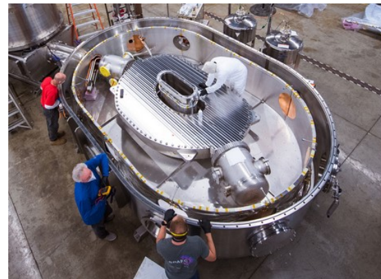
CFS – SPARC Test coil (~40 kA – ~12 T – REBCO) [1]
