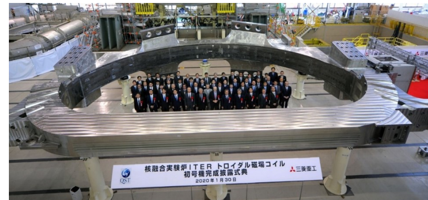
ITER – 1 st Toroidal Field Coil (68 kA – 5.3 T – Nb 3 Sn) [3]
