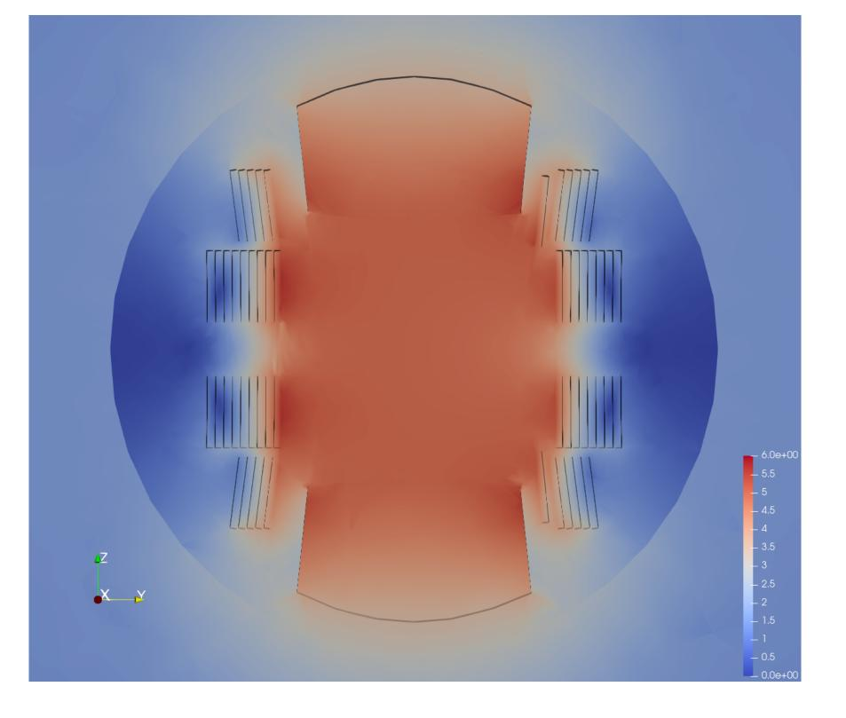
The center cross-section of field B is displayed above: a mostly uniform field is obtained in the area of interest of the magnet, with a center value of 5.02 T accurately matching the 5 T obtained in the 2D simulation of the reference thesis. While this could lead to the conclusion that a 2D analysis is enough, the cross-section in the x-y center plane below clearly indicates the need for a 3D analysis when the overall magnetic field felt by a particle is required.
