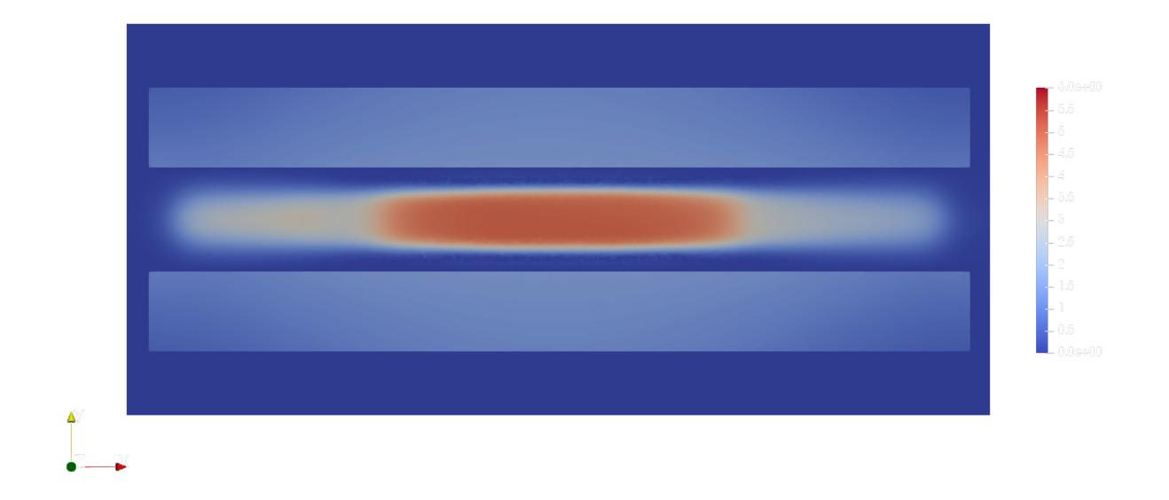
The B center value was also calculated for a sweep of supply current and is shown below. The inner iron saturation effect is visible at the slope change above a 2 kA supply current. At that stage the cylindrical core around the coils is not yet saturated and still helps further increasing B with a larger supply current.
