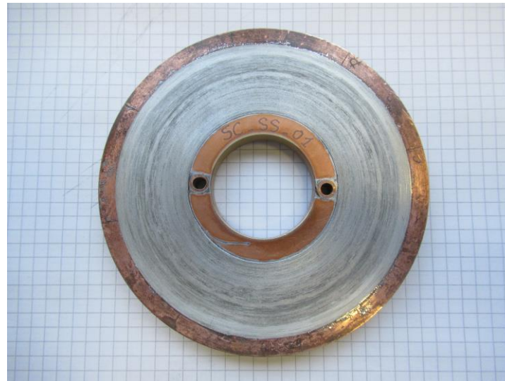
2) Single HTS tape, non-insulated, soldered
