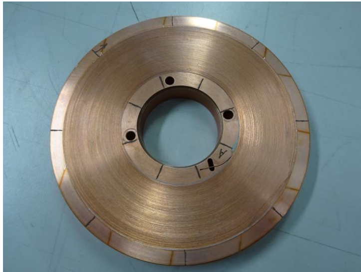
1) Single HTS tape, non-insulated, non-soldered
