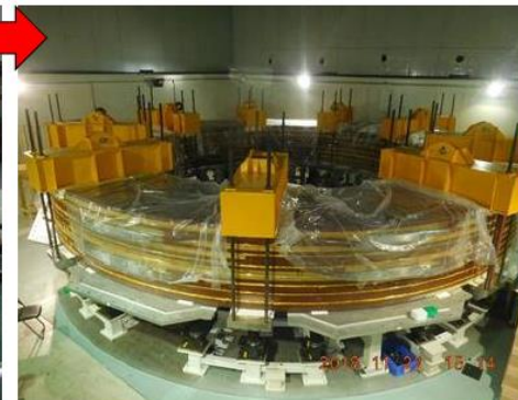
Double pancakes stacking and WP insulation
