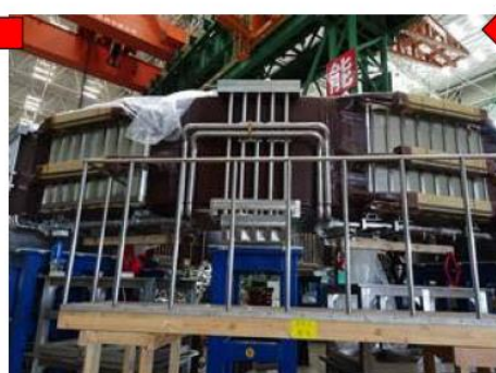
Hydraulic circuit and clamps assembly
