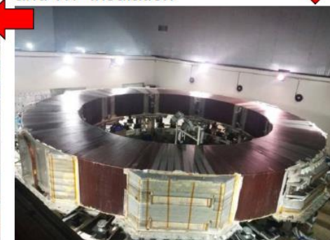
Double pancakes stacking and WP insulation
