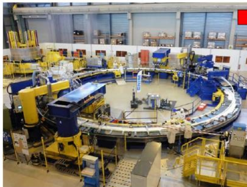
Double pancake winding and insulation
