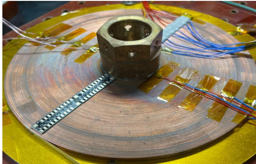
real-time field mapping of SCF in an HTS Coil using a Hall Sensor Array
