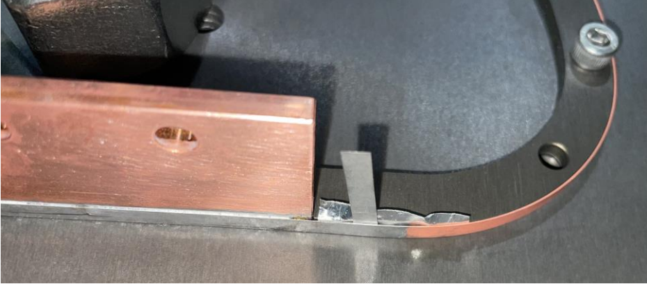
Input current lead and inner voltage tap
