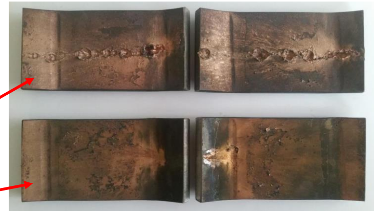
Impact traces of fragments formed in a 150 T shot.
