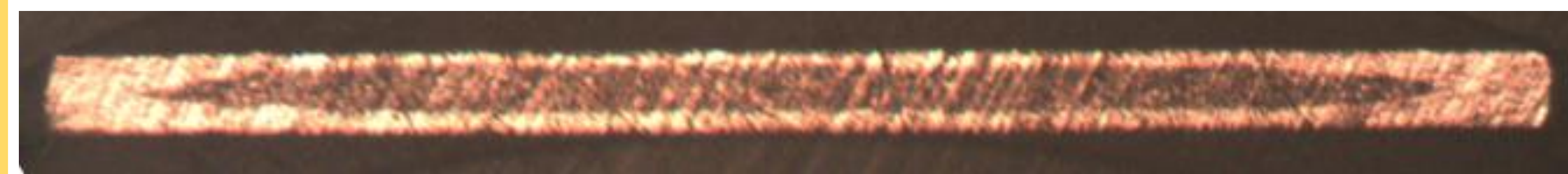
Hypertech high-C p Cu tape w/30% vol. Gd 2 O 3
