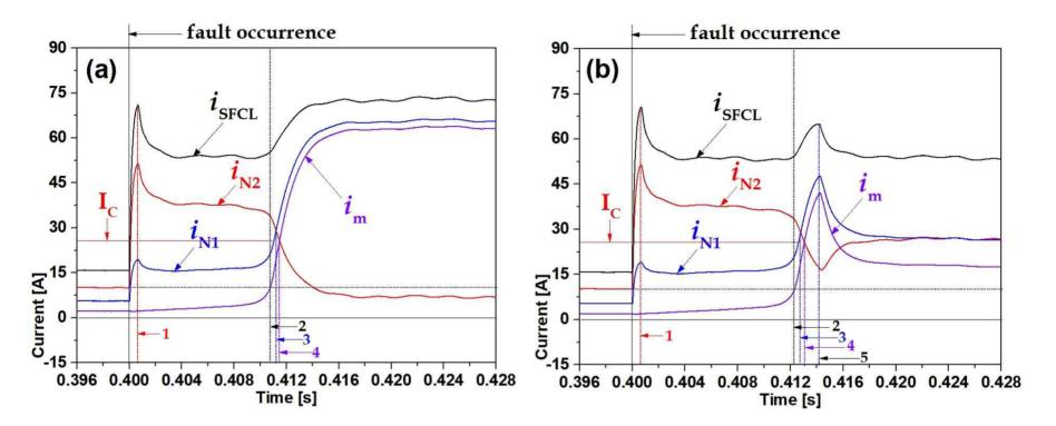
DC current waveforms depending on the number of superconducting modules of flux-locked type SFCL with subtractive polarity winding and parallel connection between two coils. (a) When one superconducting module ( $R_{sc1}$ ) is operating due to SW<sub>1</sub> ON and SW<sub>2</sub> OFF. (b) When two superconducting modules ( $R_{sc1}$ ,  $R_{sc2}$ ) are operating due to SW<sub>1</sub> OFF and SW<sub>2</sub> ON.
