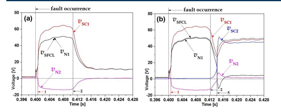
DC voltage waveforms depending on the number of superconducting modules (SMs) of flux-locked type SFCL with subtractive polarity winding and parallel connection between two coils. (a) When one superconducting module ( $R_{sc1}$ ) is operating due to SW<sub>1</sub> ON and SW<sub>2</sub> OFF. (b) When two superconducting modules ( $R_{sc1}$ ,  $R_{sc2}$ ) are operating due to SW<sub>1</sub> OFF and SW<sub>2</sub> ON.
