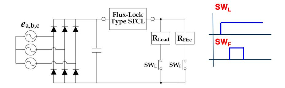
Experimental circuit diagram for DC fault current limiting test of flux-lock type SFCL with parallel connecting between two coils
