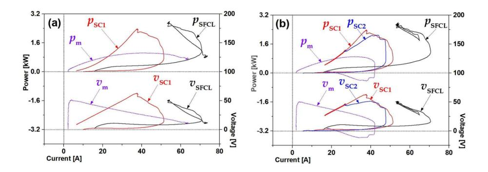
Tracks of instantaneous powers ( $p_{SFCL}$ ,  $p_{SC}$ ,  $p_m$ ) and DC voltages relationship curves depending on the number of superconducting modules (SMs) of flux-locked type SFCL during DC fault current limiting and recovery operation. (a) When one superconducting module ( $R_{sc1}$ ) is operating due to SW<sub>1</sub> ON and SW<sub>2</sub> OFF. (b) When two superconducting modules ( $R_{sc1}$ ,  $R_{sc2}$ ) are operating due to SW<sub>1</sub> OFF and SW<sub>2</sub> ON.
