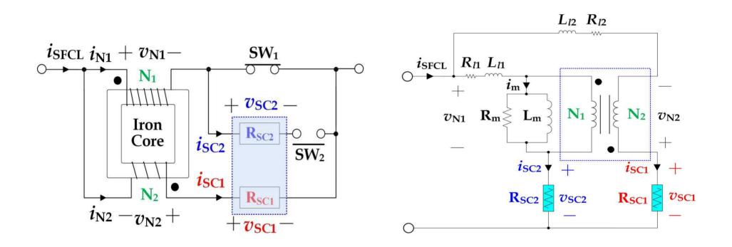
Schematic diagram of DC flux-lock type SFCL with parallel connection between two coils. (a) Structure (b) Equivalent circuit.
