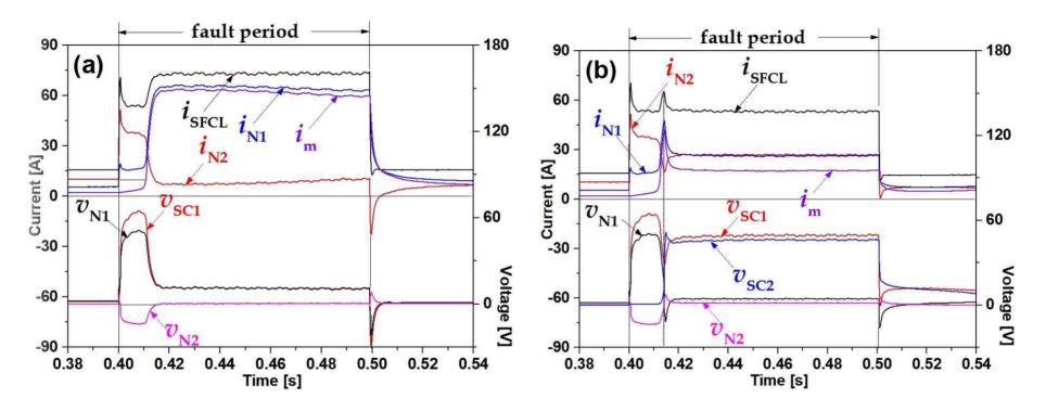
Voltage and DC fault current limiting relationship curves depending on the number of superconducting modules (SMs) of flux-locked type SFCL with subtractive polarity winding and parallel connection between two coils. (a) When one superconducting module  $(R_{sc1})$  is operating due to SW<sub>1</sub> ON and SW<sub>2</sub> OFF. (b) When two superconducting modules  $(R_{sc2})$  are operating due to SW<sub>1</sub> OFF and SW<sub>2</sub> ON.
