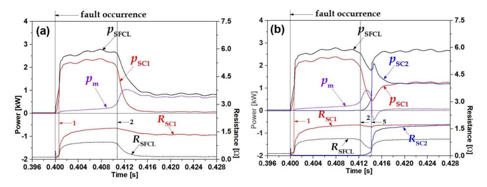
Instantaneous power and resistance relationship curves depending on the number of superconducting modules (SMs) of flux-locked type SFCL with subtractive polarity winding and parallel connection between two coils. (a) When one superconducting module  $(R_{sc1})$  is operating due to SW<sub>1</sub> ON and SW<sub>2</sub> OFF. (b) When two superconducting modules  $(R_{sc2})$  are operating due to SW<sub>1</sub> OFF and SW<sub>2</sub> ON.
