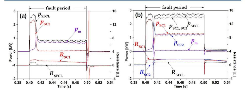
Power consumption of each devices including SMs and resistances relationship curves depending on the number of superconducting modules (SMs) of flux-locked type SFCL with subtractive polarity winding and parallel connection between two coils. (a) When one superconducting module ( $R_{sc1}$ ) is operating due to SW<sub>1</sub> ON and SW<sub>2</sub> OFF. (b) When two superconducting modules ( $R_{sc1}$ ,  $R_{sc2}$ ) are operating due to SW<sub>1</sub> OFF and SW<sub>2</sub> ON.
