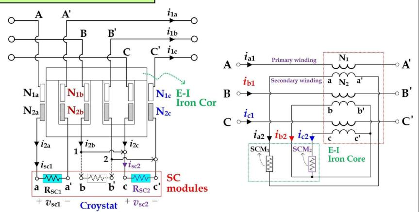
Schematic configuration of Schematic structure of three-phase transformer type SFCL using two SCMs between secondary windings
