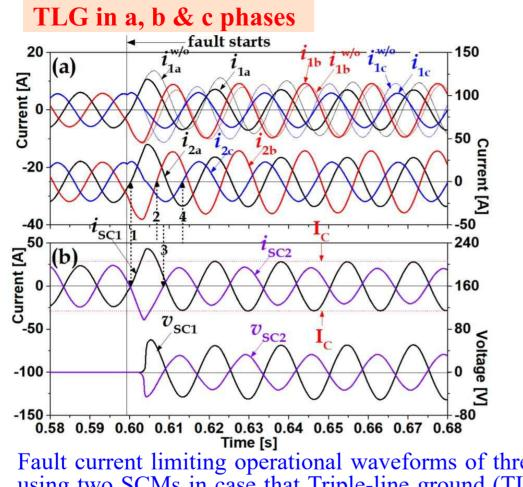
Fault current limiting operational waveforms of three-phase transformer type SFCL using two SCMs in case that Triple-line ground (TLG) fault (a) Current waveforms flowing into the primary windings  $(i_{1a}, i_{1b}, i_{1c})$  and from the secondary windings  $(i_{2a}, i_{2b}, i_{2c})$ . (b) Current  $(i_{SC1}, i_{SC2})$  and voltage  $(v_{SC1}, v_{SC2})$  waveforms of two SCMs.
