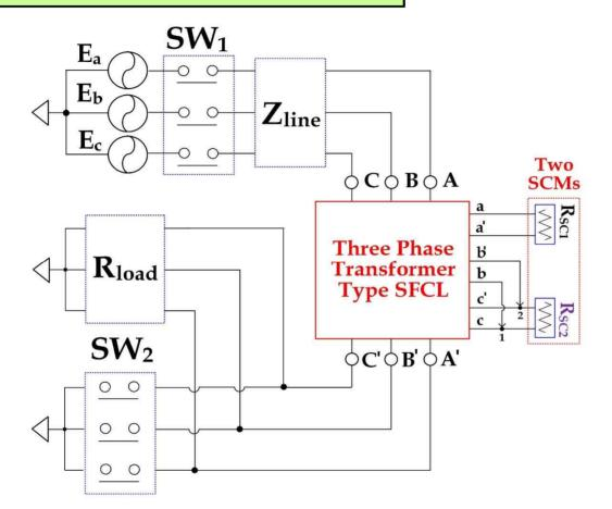
Experimental test circuit of three-phase transformer type SFCL using two SCMs between secondary windings.
