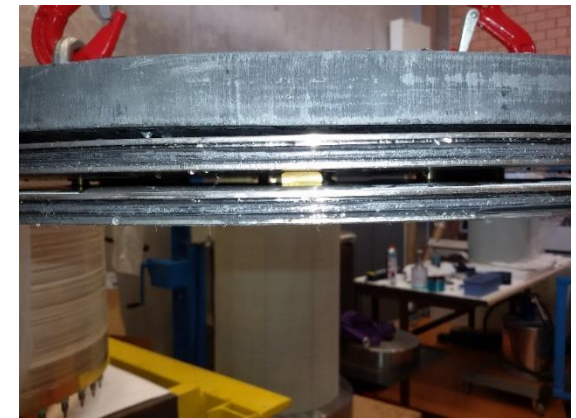
Mock-up test hydraulic bellow
