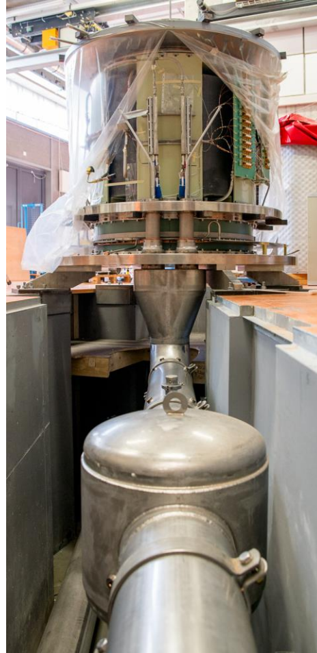
Mounted & electrically connected superconducting Al-stabilized NbTi bus bar
