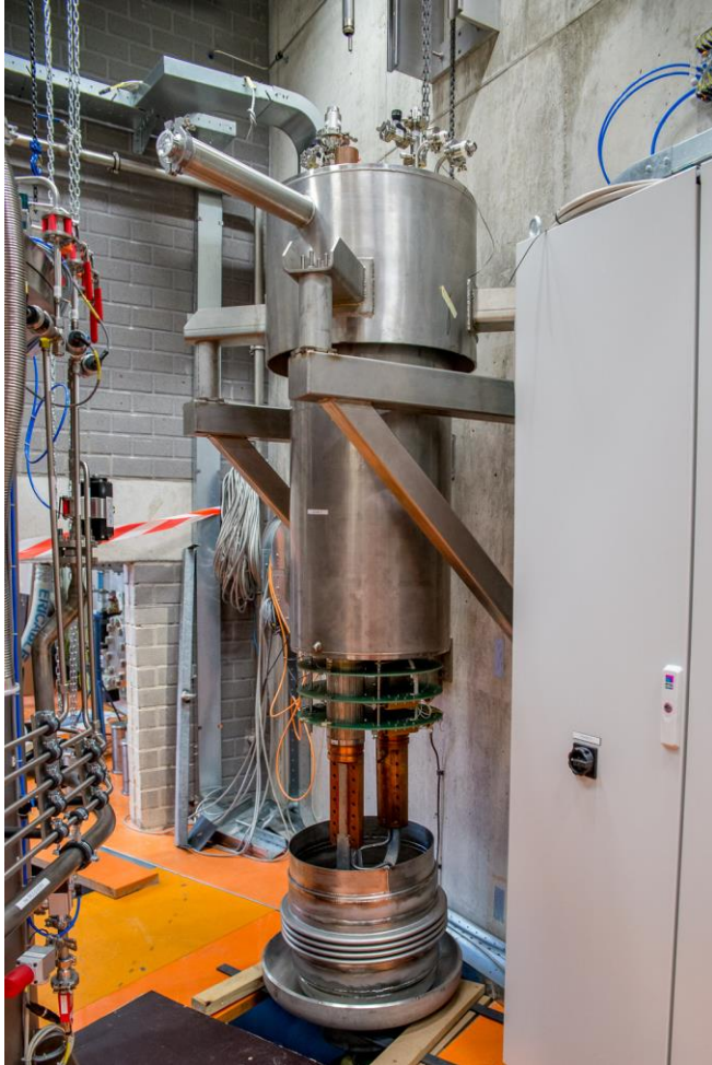
Mounted & electrically connected current lead cryostat
