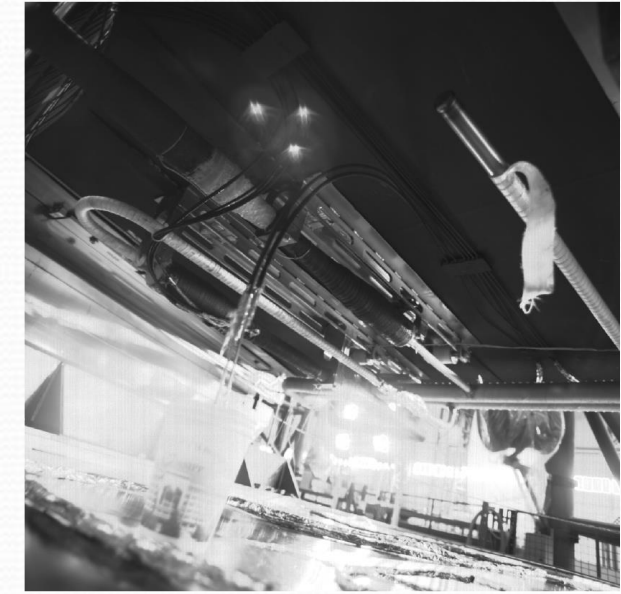
Paschen Test on PF6: HV wire exit failure
