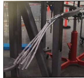
Conductor strands after chrome striping
