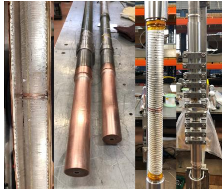
Disassembly and re-assembly of indium joint
