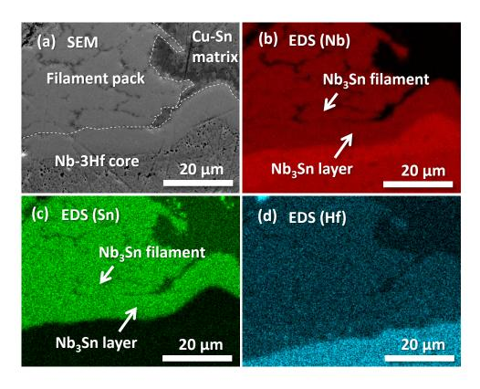
Boundary between Nb<sub>3</sub>Sn and Nb-3Hf
