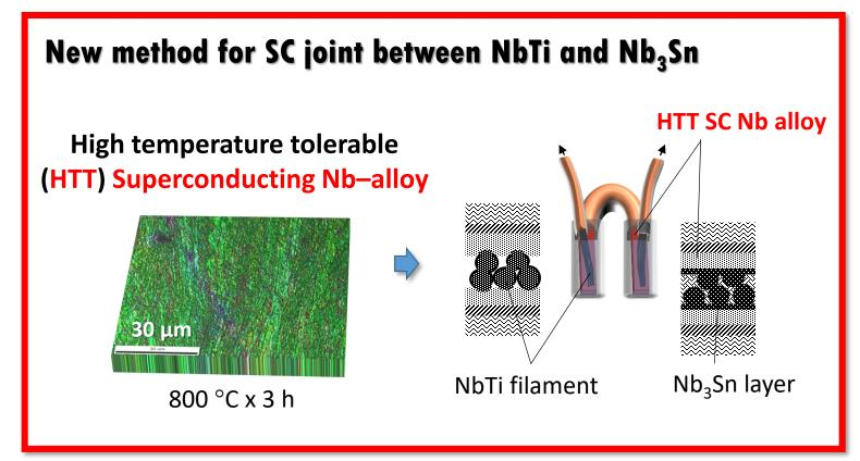
The key point is to use a high-temperature-tolerable (HTT) superconducting Nb-alloy as an intermedia, whose critical current does not deteriorate even after exposure to temperatures higher than 650 °C.
