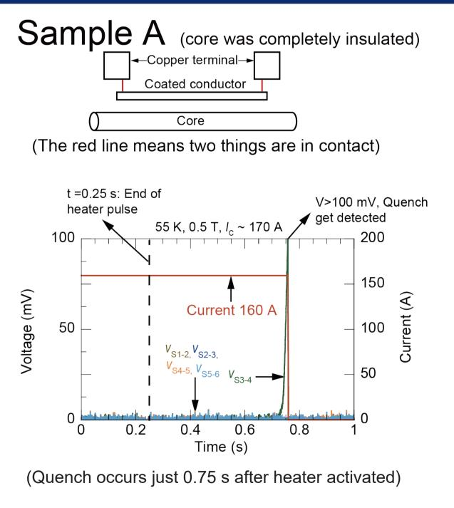
The hot-spot temperature of spiral coated conductors using metal core is much lower than those with heatinsulating core (e.g., GFRP core).
