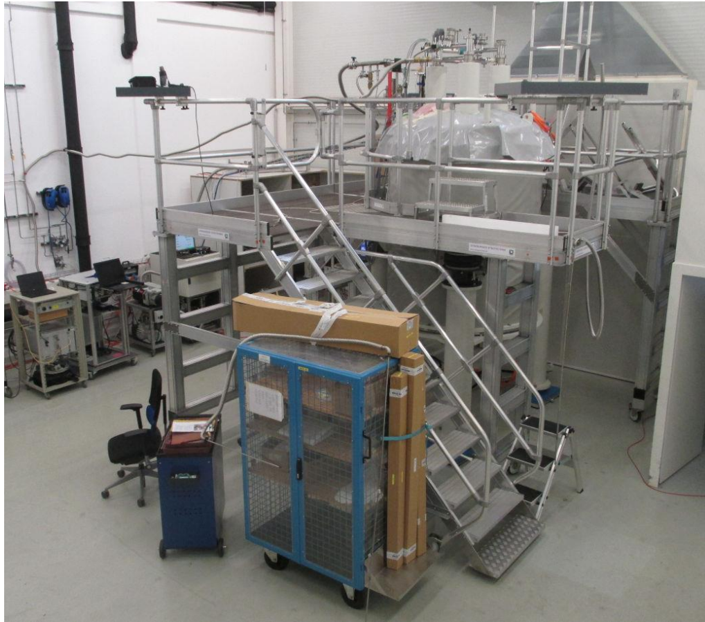
On this test stand the first 1.2 GHz magnet reached field
