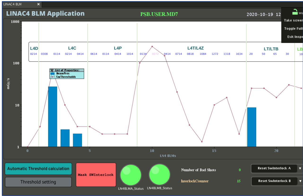
Tuning of SW Interlock Thresholds in LN4
