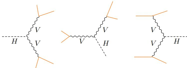
HVV couplings can be probed in  $H \rightarrow VV$  decays and  $VH$  and  $VBF$  production modes: four-fermion kinematics is sensitive to the HVV coupling structure.
