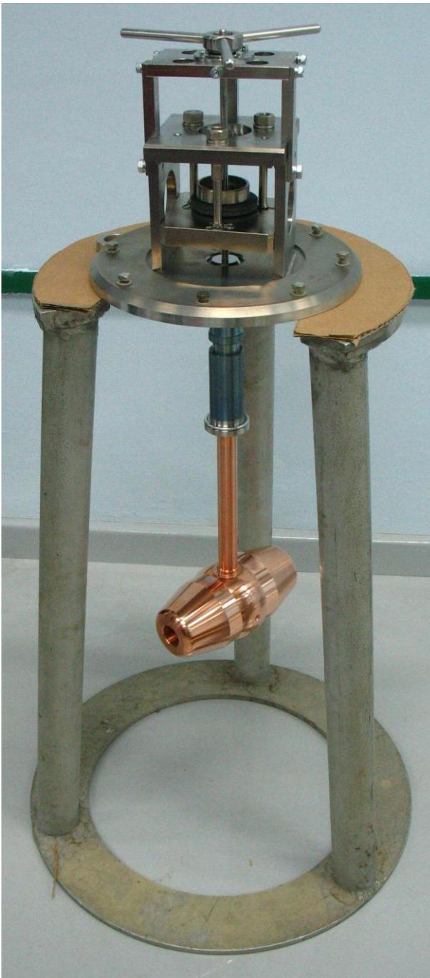
Drift tube mock up built at BINP passed dimension check, vacuum leak check and water pressure (up to 16 bars) check
