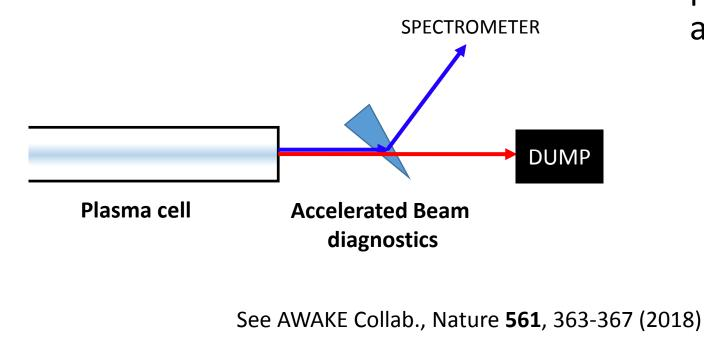
The electrons are captured in the plasma wakefield and accelerated after the self-modulation
