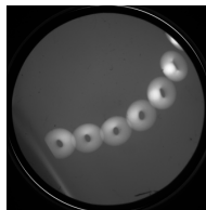
Figure: Camera image of six beam spots captured at a phosphor screen 67 cm downstream of the prototype Gabor lens.
