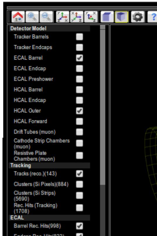
A screenshot of the CMS detector model interface. It features a toolbar with icons for home, search, zoom, and other functions. Below the toolbar is a list of detector components with checkboxes:
