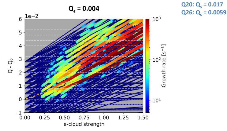
The effect of the synchrotron tune has been studied with bunch intensity  $N_b = 2 \times 10^{11}$
