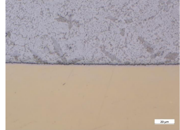
interface between the connector and the solder
