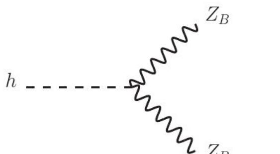
Feynman diagram illustrating the decay of a Higgs boson ( $h$ ) into two  $Z_B$  bosons. A horizontal dashed line represents the Higgs boson, which decays into two wavy lines labeled  $Z_B$ .
