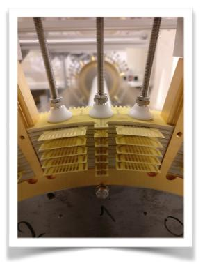
Innovative wire techniques (no feedthrus) Very <u>fragile</u>, sensitive to humidity and contaminants
