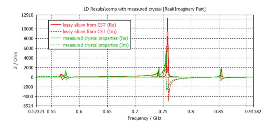
→ Frequency shift of 2.5 MHz and reduction of the crystal mode by a factor 2.4
