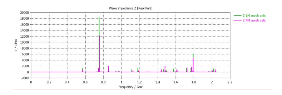
Im(Z/n)~1 mOhm (i.e. ~1% of the total LHC low frequency until 500 MHz) for 1 crystal
