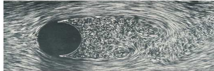
(b) a closer look at Re = 2000 - patterns are identical as in (a) [Courtesy: ONERA pic. Werle & Gallon (1972) from An Album of Fluid Motion by van Dyke (1982)]
