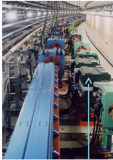
Replace short dipoles with longer ones (LER)
