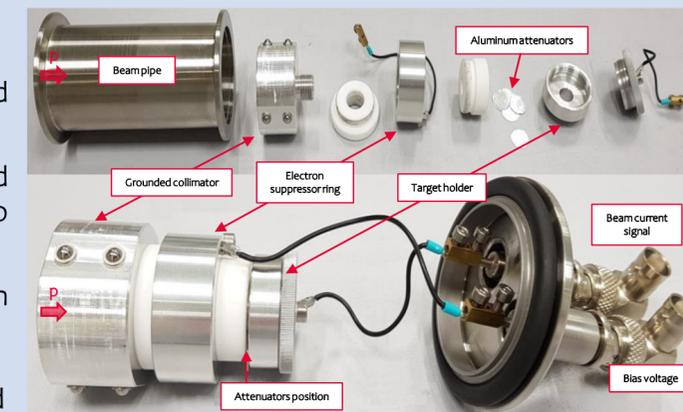
Aluminum attenuator discs can be located in front of the target to modulate the energy of the impinging protons.
