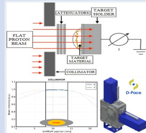
The number of protons per unit area hitting the target is determined by measuring the current in real time during the irradiation, thanks to a customized target station.
