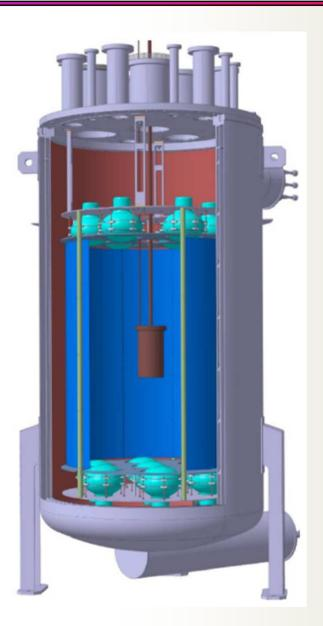
OFHC copper vessel with two top pipes. Total weight → 7 kg and volume → 3 L.
