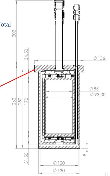
OFHC copper vessel with two top pipes. Total weight  $\rightarrow$  7 kg and volume  $\rightarrow$  3 L.
