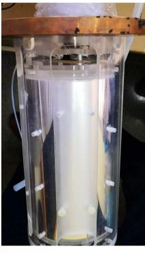
• Reflector around SiPMs and between acrylic cylinders.
