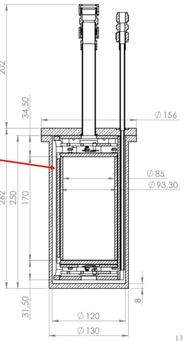
OFHC copper vessel with two top pipes. Total weight → 7 kg and volume → 3 L.
