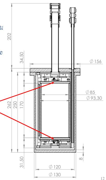
OFHC copper vessel with two top pipes. Total weight  $\rightarrow$  7 kg and volume  $\rightarrow$  3 L.
