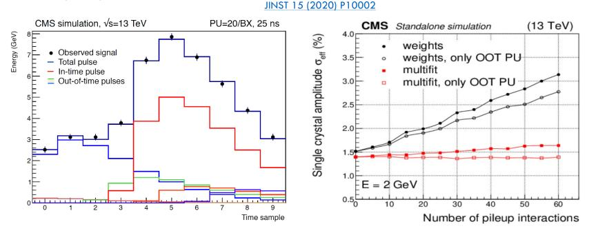
The 'multifit' reconstruction method is robust against pileup increase.
