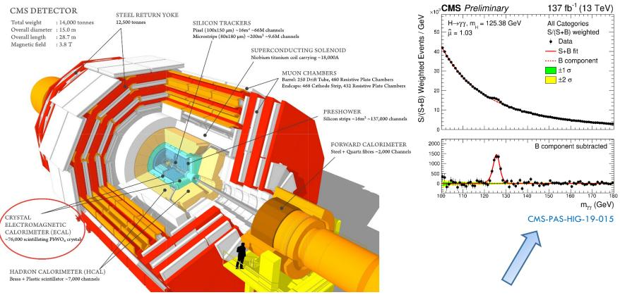
The electromagnetic calorimeter plays a crucial role in many CMS physics analysis that involve electrons or photons
