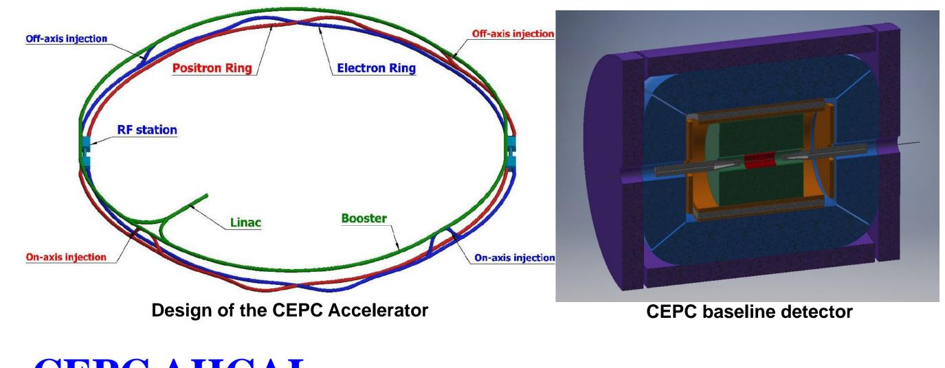
• CEPC AHCAL simulation: The scintillator-steel AHCAL is implemented into the CEPC detector geometry. A particle flow algorithm named arbor is used to reconstruct the H-gg events. The Higgs boson mass resolution(BMR) is required to be less than 4% for the benefit of CEPC physics. Detector parameters like: absorber thickness, sampling layers, scintillator thickness and cell size, have been scanned to optimize the BMR. The results is found to be consistent with the prototype design
