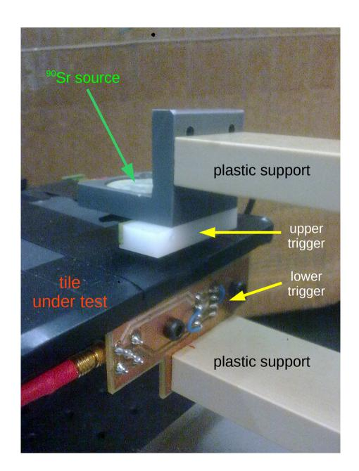
the trigger is given by a small telescope (2 x 1cm scintillators)
