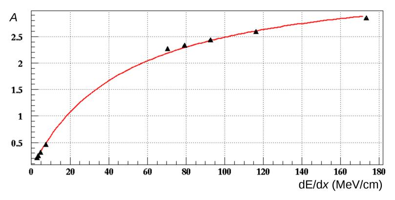
The correlation between the signal amplitude and the dE/dx is well fitted with a Birks' law (provided the SiPM are not saturated)
