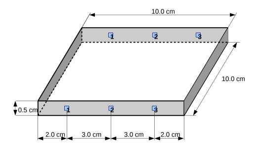
Test performed on a 10x10x0.5 cm<sup>3</sup> plastic scintillator tile (EJ200 type)
