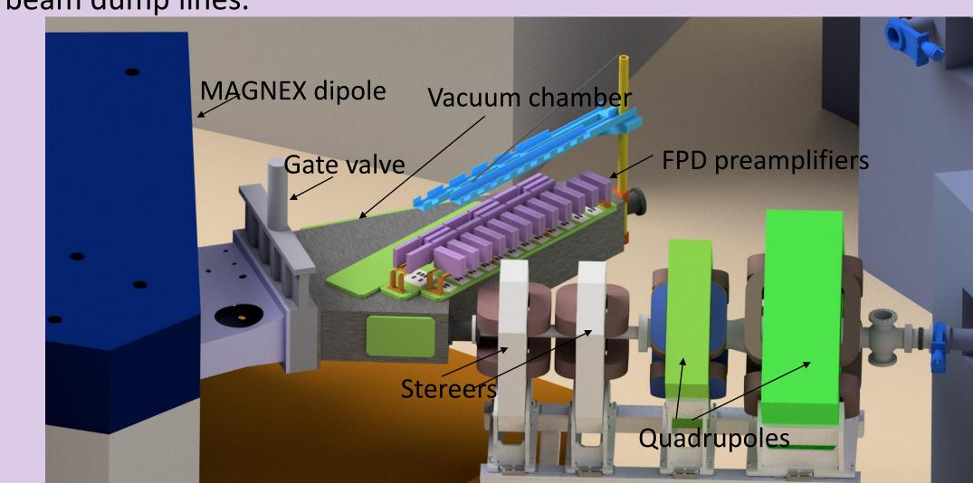
The FPD, tilted with an angle of 59° with respect 18 O beam line 20 Ne beam line the gate valve shutter, is positioned in the middle and filled with isobutane (absolute pressure of pprox20 mbar). It offers a few µm thin mylar window (920 mm x 150 mm) to the entry of ions coming from the vacuum part of the chamber.
