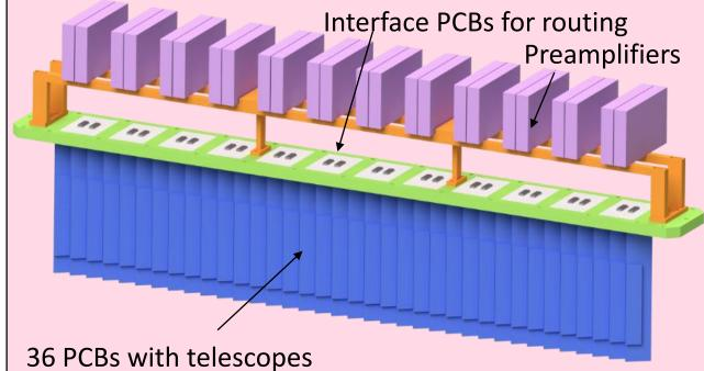
Preamplifiers A custom PCB houses 20 telescopes, 10 row and two columns 36 cslboards build the PID wall, each tilted of 35° angle with respect the frame tracker
