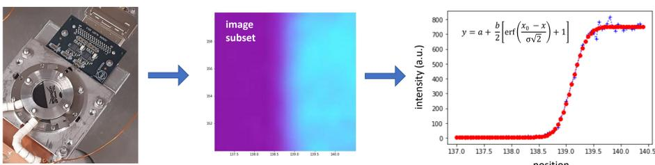
The spatial resolution of the detection module was determined with the edge spread function method. An image of a sharp edge was obtained with a positron beam of 0.5 keV. The image intensity along the edge is integrated and fitted with an error function. The resolution is extracted from the parameters of the fit.
