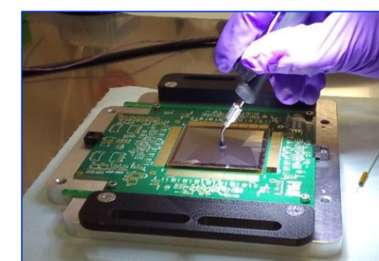
Strip X detector assembly in INFN – Perugia Clean Room
